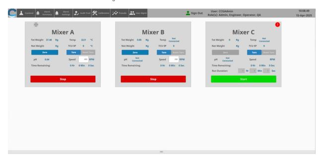
When Temperature or pH instruments are connected, real-time process variables are displayed for the channel in which they're connected (A/B/C)
